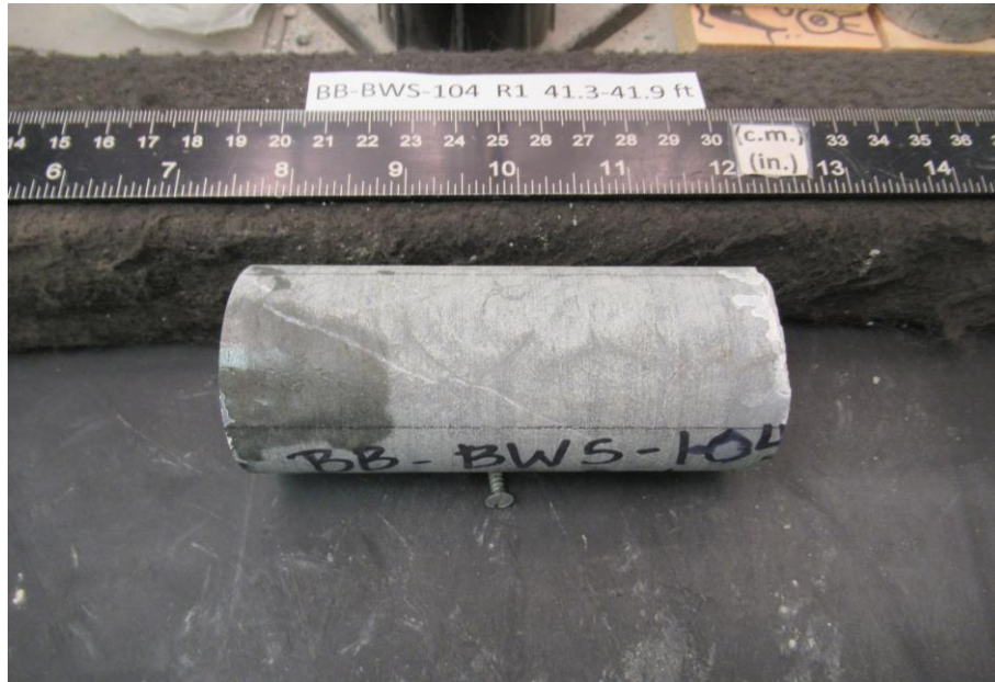
After cutting and grinding
